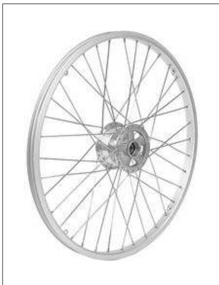
C2. Standard wheel with drum brake
