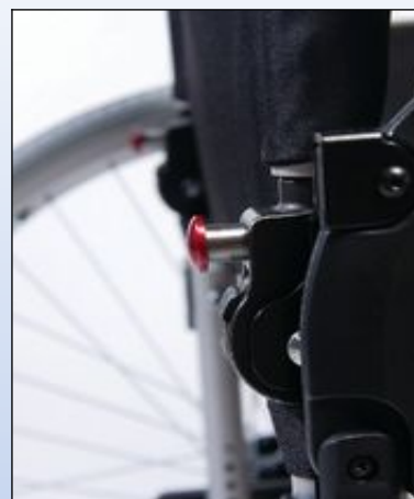
HY1c. Detail of the release button of the tilting mechanism
