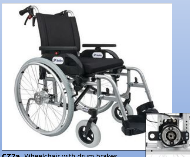
CZ2a. Wheelchair with drum brakes
