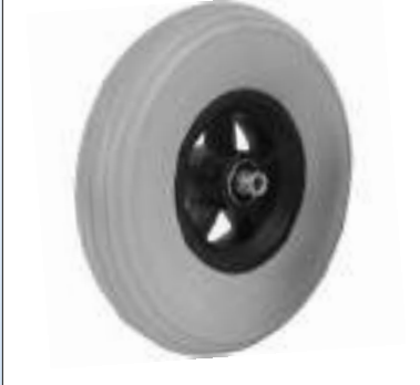
8" Flexel wheel, 200 x 50, off-set hub Ø12 x 60 mm
