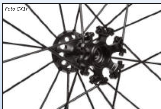
Spinergy CNX milled hub 2,30", 1/2" bearings, red or black for XSLX wheel
