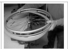
3. Put the PU tire on the wheel and push the tire as far as possible into the rim. Make sure that the vertical fin is located between tire and rim.
