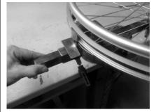
2. Move the sliding carriage on the PU fitting device so that the vertical "shark fin" easily applies to the rim and fix the sliding carriage with the star screw.
